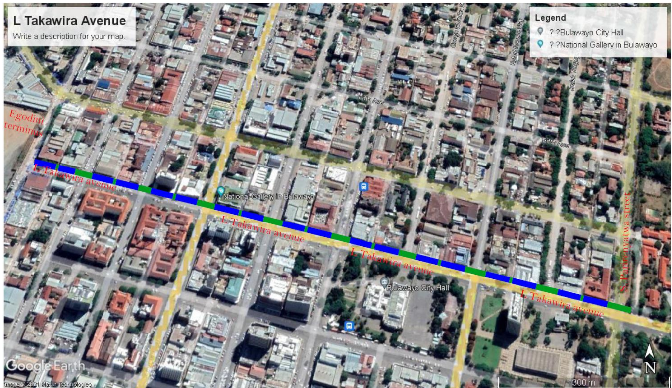
Figure 7: The proposed tactile street roof along Leopold Takawira Avenue. Blue shows the canopy system and green is the extension over streets and service lane.
